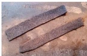
Fig.4 Tanned leather specimen for determination of shrinkage temperature
