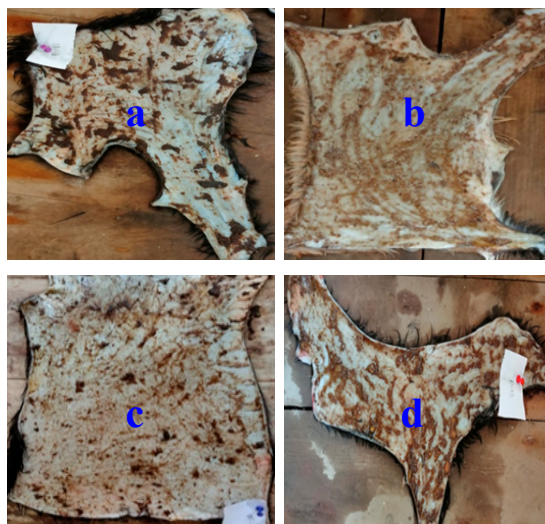
Fig.2 Application of 5% banana peel paste with 10% salt (a) 10% banana peel paste with 10% salt (b) 15% banana peel paste with 10% salt (c) and 20% banana peel paste with 10% salt (d)
