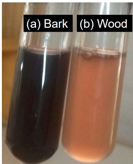
Fig.2 Ferrous sulphate reagent test. Indicated presence of (a) Catechol in bark and (b) pyrogallol in wood
