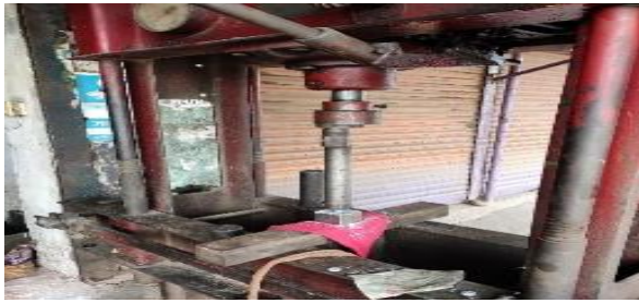
Fig. 9: Compaction of powder mixture in a hydraulic press
