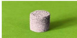
Fig 11: Magnesium oxide foam of wt% 55-45 of MgO and NH 4 HCO 3
