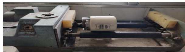
Fig. 8: Ball milling of magnesium oxide powder and space holder
