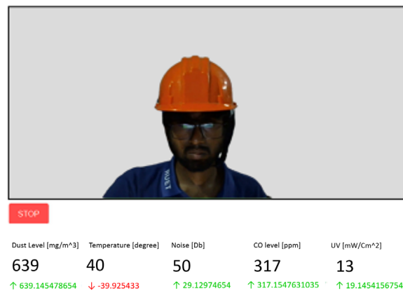
Fig 6: Dashboard of the monitoring system.
