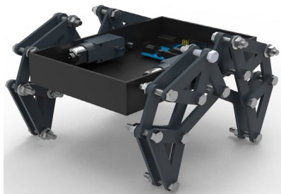
Fig.1 CAD model of a four-legged walking robot using Theo Jansen Mechanism.
