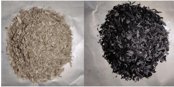
Fig.2 Raw Jute Stick Powder (at left) and Produced Charcoal after Carbonisation (at right)
