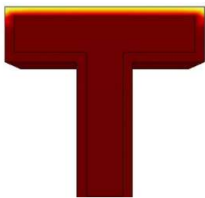
Fig.6 Heat Propagation through T-bar with Coating
