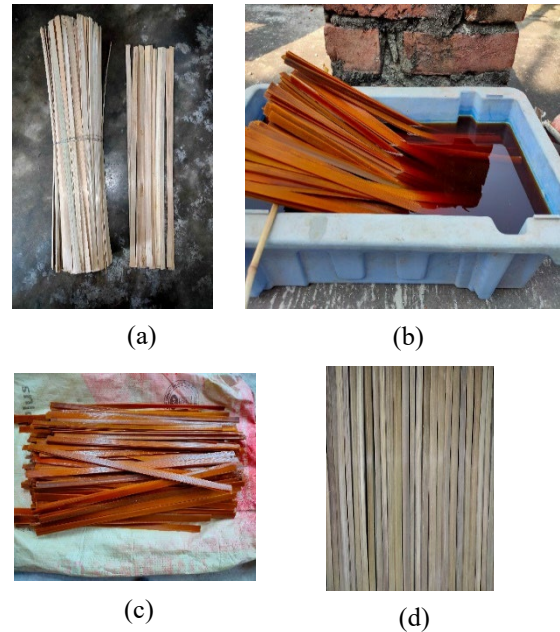
Fig.2 (a) Untreated bamboo strips, (b) Alkaline treatment, (c) Bamboo strips after alkaline treatment, (d) Bamboo mat.
