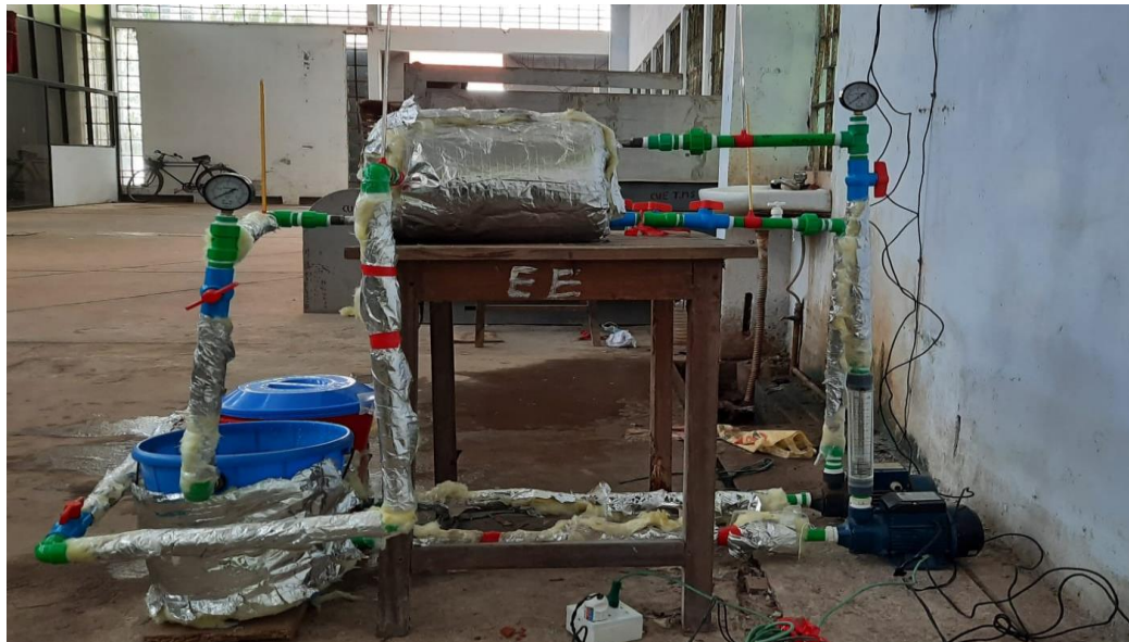
Fig. 4 Photographic view of the experimental setup of shell and helical coil heat exchanger.
