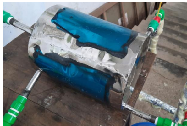
Fig. 2 Fabricated helical coil and shell heat exchanger.
