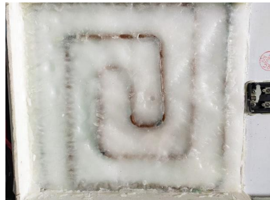
Fig. 2: Photographic view of commercial grade paraffin wax with copper pipe layout
