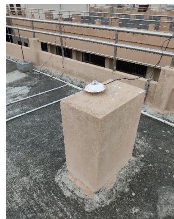
Fig.5 Measurement of global solar radiation by a pyranometer.
